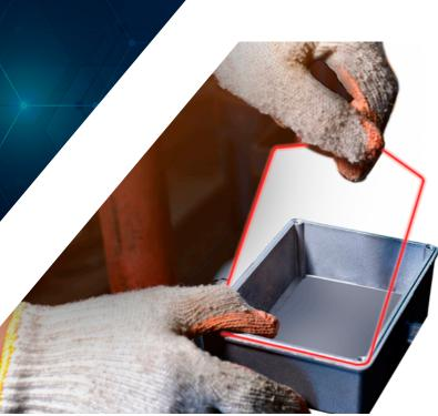
For water and dust proofing applications, moulded and cut gaskets are widely used. These gaskets are typically assembled by hand.
